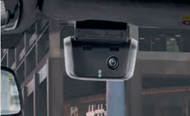
Advanced Car Eye 2.0. A highly sensitive full-HD camera that captures events in front of and behind the car, even when it is parked. In the event of disturbances and extraordinary movement outside the vehicle, the camera automatically records the situation in order to document possible accidents or (attempted) break-ins.
