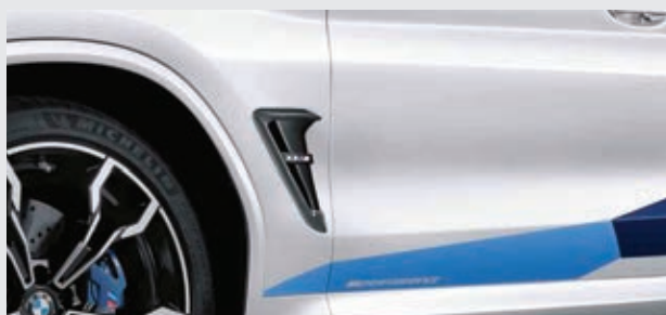
M Performance Air Breather in Carbon Fibre. Visual highlight on the side of the vehicle: The BMW M Performance Air Breather is made of premium carbon fibre.
