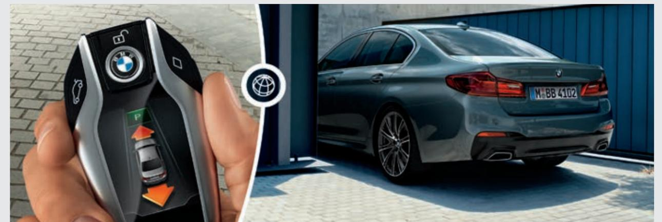
**Remote Control Parking with BMW Display Key** function allows the driver to conveniently get out of the vehicle before parking it via remote control by moving it forward into, or reversing out of a tight parking space or garage. The driver activates the remote-controlled parking function from outside the vehicle via the BMW Display Key.
