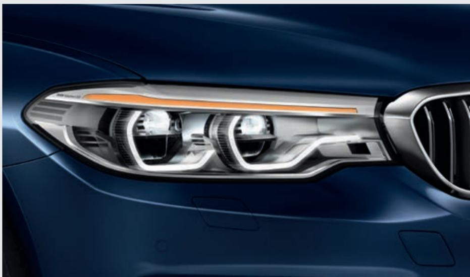
The **Adaptive LED Headlights with High Beam Assistant** include BMW Selective Beam, cornering lights and adaptive headlights. The light colour is similar to daylight and provides an ideal, even illumination of the road to improve visibility and make driving in the dark less tiring.
