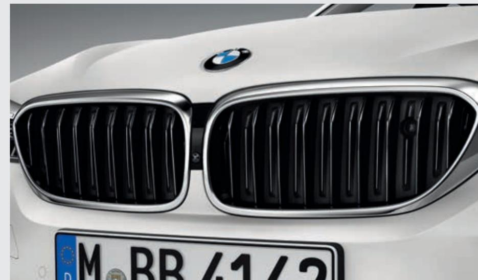
The **Active Air Stream Kidney Grille** knows when the engine, brakes and other components need air and automatically opens the air vents. If no further air intake is required, it closes them again. This improves aerodynamics and fuel consumption falls.
