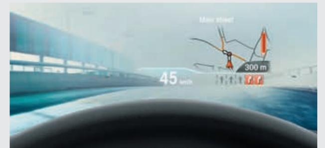
The **BMW Head-Up Display** offers a full-colour projection of driving relevant and situational information onto the windscreen with improved resolution of 800 x 400 pixels.
