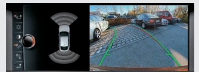
The **Reversing Assist Camera** enables improved orientation when reversing at speeds below 10 kmph. It shows the area behind the car on the Control Display. Interactive track lines for measuring distance and turning circles assist the driver when manoeuvring, obstacles are marked in colour.
