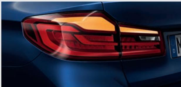
The **LED Rear Lights** are split into two parts, with LED technology featured in the tail lights, brake lights, turn indicators and reversing lights.
