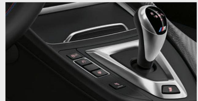
□ Shift gears without losing power, using the clutch or slowing down: the 7-speed M double-clutch transmission with Drivelogic. Gears can be changed automatically or manually using the gearshift paddle switches on the steering wheel, or the gear selection lever. Launch Control guarantees maximum acceleration from a standing start.
