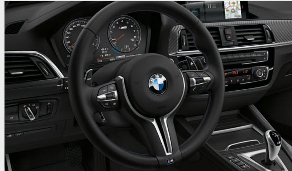
■ Depending on the equipment, Multifunction for steering wheel can be used to operate the telephone, voice control and audio functions via the buttons on the steering wheel. The Manual Speed Limiter is also integrated. It can be used to set an upper limit of 50 km/h for city driving, for example.
