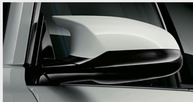
■ The aerodynamically optimised M exterior mirrors are a significant part of the sporty and dynamic M design. Attached to the body by a double-bridge designed base, they underscore the beautiful aesthetics of the car and convey a sense of precision engineering down to the last detail. The additional LED indicators are fitted perfectly into a long, narrow groove.
